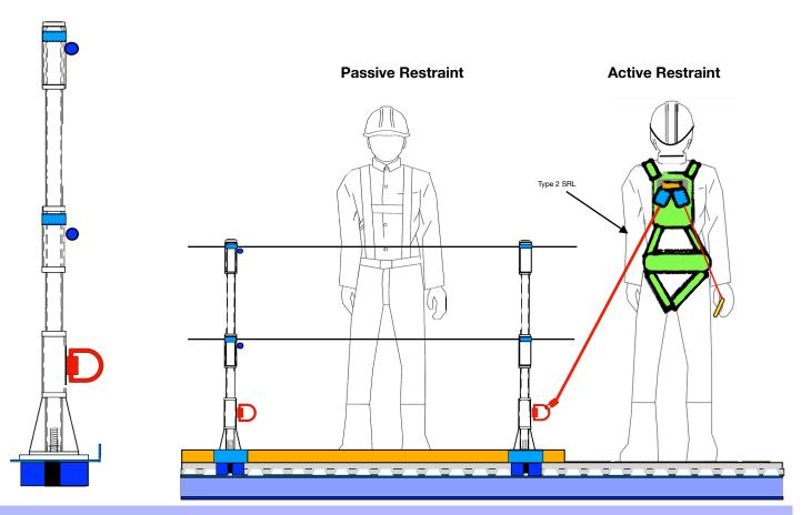
SAP42DM Requires: CLT3 anchor welded to structural steel (100% tie-off) without wire-rope; (100% reusable) Compare
