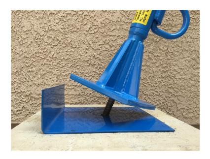
Grease coil-rod from SAP post with Lithium White grease prior to installation.
