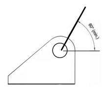
Minimum sling for the rigging is  $45^{\circ}$  from horizontal. We recommend using a sling angle of  $60^{\circ}$  if lifting headroom is not an issue.
